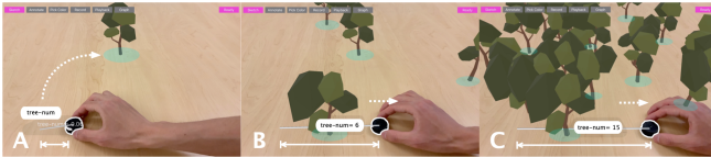
Figure 22. Tracked object parameters can be mapped to a program property through a pre-defined variable name. In this case, the number of virtual trees is controlled by a tangible slider.
