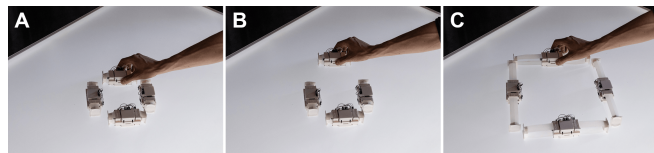
Figure 17. Interactive shape change. A) A small rectangle shape. B) If the user moves one element, C) then the robots change positions and lengths to scale the square.
