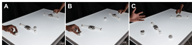
Figure 20. Tangible game controllers. A) Two user start playing a table football game. B) Each user uses one ShapeBot as a controller and another ShapeBot to hit the ball. C) The user can play with these ShapeBots like table football.
