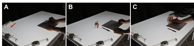
Figure 21. Shape-changing Tools. A) A user is working on a desk. B) When the user needs a pen, ShapeBots can bring it. C) ShapeBots can be also used as a tool like ruler.
