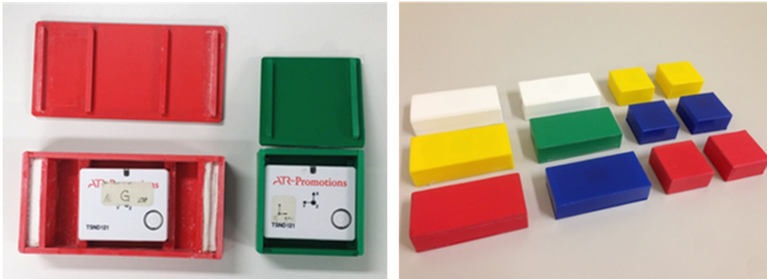
Fig. 3. Toy blocks with the embedded Bluetooth-IMU-sensors
