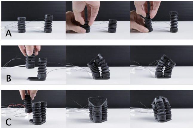
Figure 6. By combining multiple MorphIO modules, we can achieve higher degrees of freedom for more complex deformation. Deformation using a single unit (A), two units connected in parallel (B), and three units connected in circle (C).
