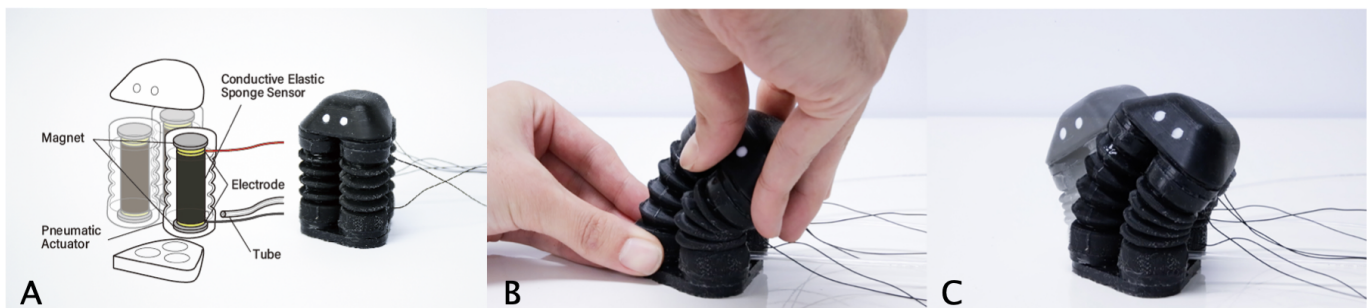
Figure 1. MorphIO is a modular and entirely soft sensing actuation unit for programming by demonstration of soft robots. (A) Each MorphIO unit consists of a pneumatic actuator containing a conductive elastic sponge sensor, which both senses and actuates three-dimensional deformation. The modular design of MorphIO's unit allows the user to construct various shapes and topologies through magnetic connection. (B) The user can demonstrate and record motion through tangible interaction. (C) The recorded motion can later be played back through pneumatic actuation.
