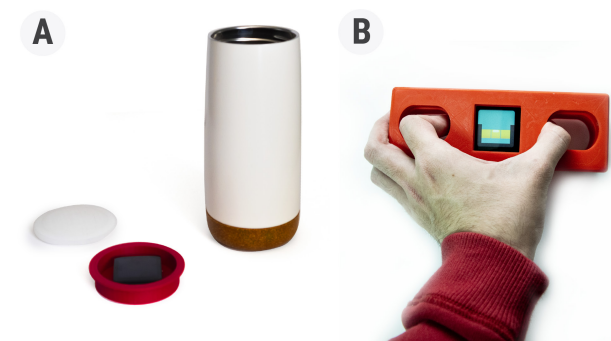
Figure 7. Our Soul-Body Prototypes working with Astral: (a) Smart Speaker, prototyped by 3D printing a watch tray and light diffuser fitted inside a travel mug; (b) 3D Printed ‘Smart’ Level that reuses our phone app on an enclosed smartwatch.
