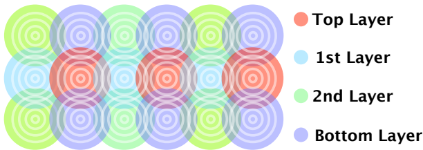
Figure 8. A simplified schematic of our coil design of a 4-layer PCB. Each layer has a set of coils aligned with a certain offset in both horizontal and vertical directions. Each coil is 15 mm diameter and has 2.5 mm overlap between nearby coils.
